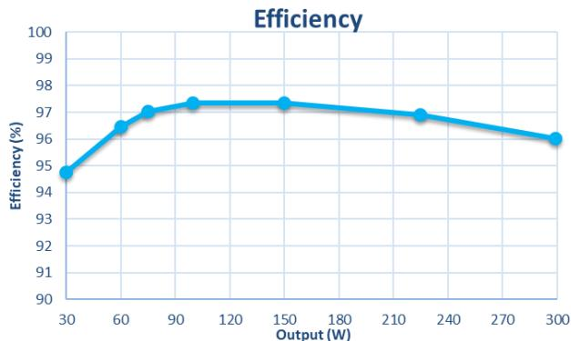
Fig. 9 the efficiency of LLC converter
